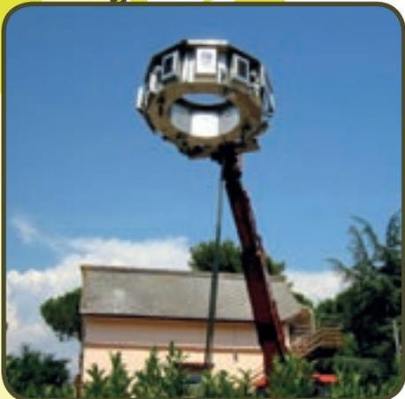
**ECOPALM Ring** is a device built as **CIRCULAR BAND**, endowed with electric generators of microwaves that radiate the high frequency energy toward the center of the palm tree. The device is endowed with sectors that **OPEN** and **CLOSE** electrically for the insertion of the palm tree to treat inside the circular band.
